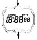
3) Finally check the connecting portions of the liquid crystal panel and the connectors.
