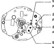
Set the small second wheel and pinion of Cal. 7N08A here.
