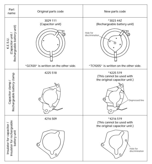
\* When you change the original capacitor to new rechargeable battery unit, the clamp and the insulator are also required to be changed. Please order them as a set by parts code <u>3023 5MZ</u> to avoid confusion. (<u>3023 5MZ</u> contains rechargeable battery unit, rechargeable battery clamp and insulator.)
