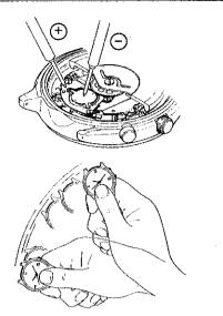
4) If the voltage obtained has increased more than 0.1V from the initial voltage, the automatic generating system is normally operating.
