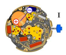
Setting stem in position I, calendar not in gear, 60 s measuring interval for rate and consumption:
