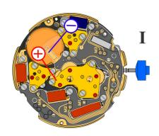
Setting stem in position I, calendar not in gear, 60 s measuring interval for rate and consumption:
