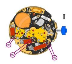
1.90 k $\Omega$  .. 2.10 k $\Omega$ Coil resistance M1
