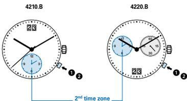
Any 2nd time zone can be set using the small hour hand and small minute hand.
