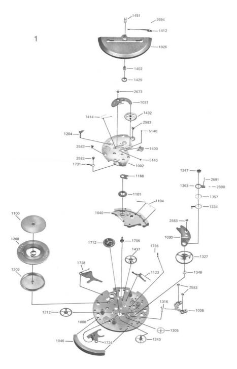
1000 Plate 1204 Barrel axle 1002 3/4 plate bridge 1005 Pallet cock 1026 Rotor 1030 Balance cock 1031 Bridge for automatic device 1040 Stem cock 1046 Rotor support 1100 Ratchet wheel 1101 Crown wheel 1104 Clicking spring 1123 Stop-lever 1168 Crown wheel lid 1202 Barrel drum
