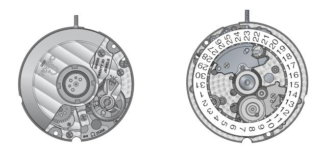
Automatic movement. Omega customised. Display of hour, minute and second in centre, date display. Swiss lever escapement.
