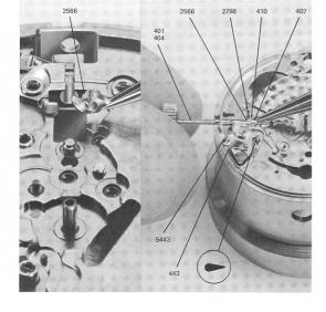
8.1.11 Take out the screw (5443). Remove in order the yoke 435, the setting lever 443, the sliding pinion 407, the winding pinion 410, the date-corrector maintaining plate 2798, the date-corrector 2566 and the winding stem 401 or 404.
