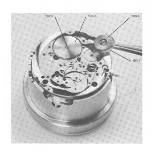
8.4.5 Fit in order the escape wheel 705, the third wheel 210 (with the pinion upwards), the fourth wheel 220 (with the pinion downwards), the center wheel 201.1 and the train bridge 110, fixing it by means of its two screws (5110). Check the endshake of the arbors.
