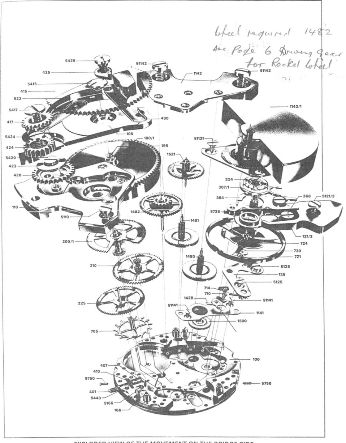
EXPLODED VIEW OF THE MOVEMENT ON THE BRIDGE SIDE
