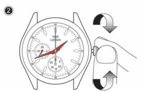
Turn the crown clockwise to set the desired time taking AM or PM into consideration.
