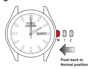
• Push the crown back to the normal position. Check the second hand begins to move.
