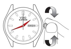
• Turn the crown to set the hour and minute hands. Set the hour and minute hands to the desired time taking AM/PM into consideration.
