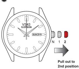
• Pull the crown out to the 2nd click position when the second hand is at the 12 o'clock position.
