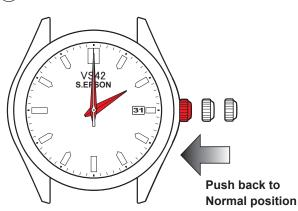
• Push the crown back to the normal position. Confirm that the second hand begins to run.
