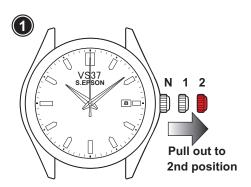
• Pull the crown out to the 2nd click position when the second hand is at the 12 o'clock position.
