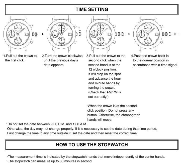
(The watch indicates the measurement time in second increments by ignoring off the 1/10 seconds obtained.)
