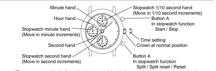
\*The measurement time indicated by the stopwatch hands that move independently of center hands. \*Stopwatch 1/10 second hand moves for a first minute.
