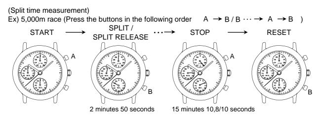
\* Measurement and release of the split time can be repeated as many times as necessary by pressing button B.
