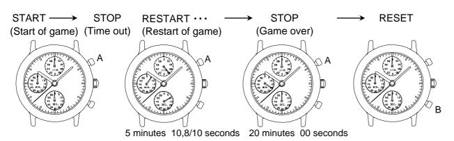
\*Restart and stop of the stopwatch can be repeated as many times as necessary by pressing button A
