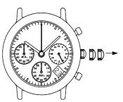
3.Pull out the crown to the second click when the second hand is at the 12 o'clock position.
