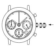
4.Push the crown back in to the normal position in accordance with a time signal.
